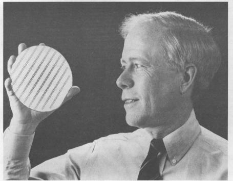
BOB BLEWER (DMTS, 2132) looks at a semiconductor wafer of the type used for making integrated circuits, or "chips." After the chips have been formed on the wafer, they are cut apart to be packaged and assembled.
